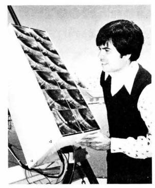
DAN ARVIZU, project leader for an experimental silicon solar cell module, checks the unit's performance at Sandia's Photovoltaic Test Facility. The state-of-the-art module tests at 17 percent efficiency — 17 percent of the solar energy falling on the module is converted directly to electricity.
